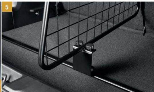
**5 | Adapter for Cargo Partition Grid (Lengthwise)** <sup>48V</sup>
